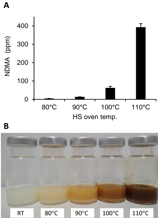
**Fig. NDMA formation in ranitidine tablet sample by 10-min heating at various temperature in Headspace-GC analysis**
