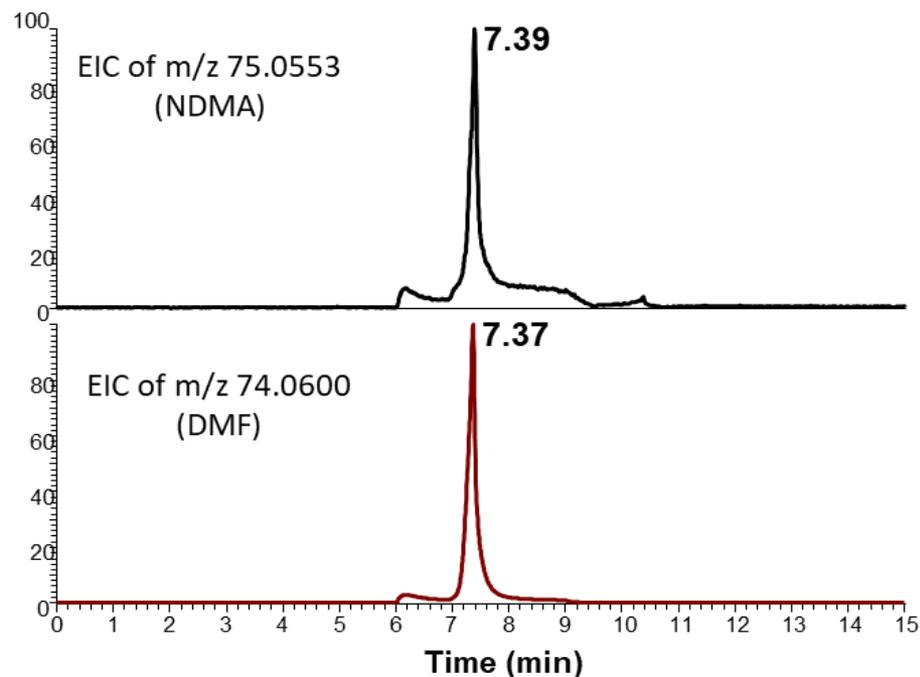
Fig. Co-elution of NDMA and DMF in the chromatography used by the private laboratory. The EIC of the exact mass of NDMA (eluting at 7.39 min) and EIC of the exact mass of DMF (eluting at 7.37 min) are indicated in the Figure.
