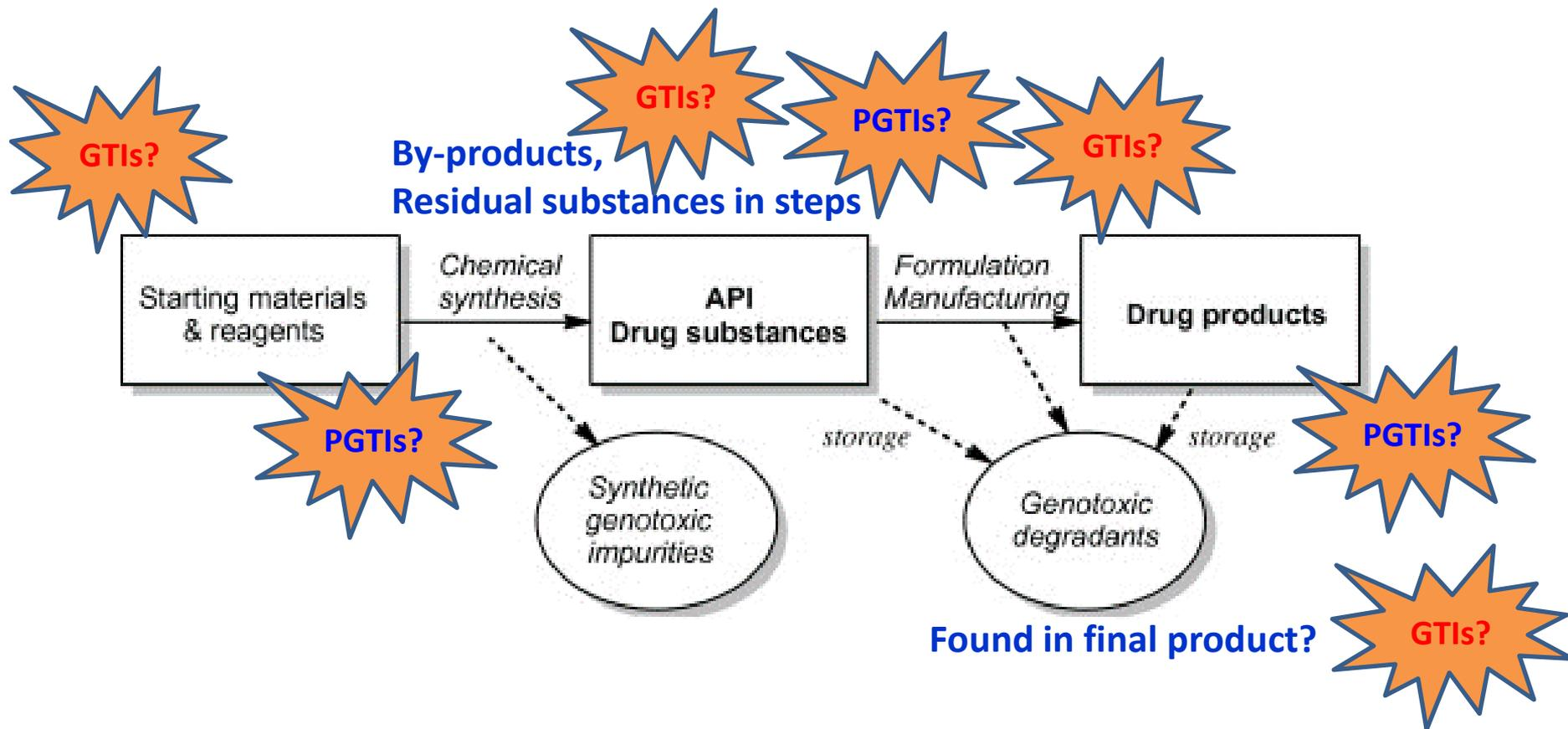
Fig. A typical chemistry and formulation process showing where synthetic genotoxic impurities and genotoxic degradants can be generated.
