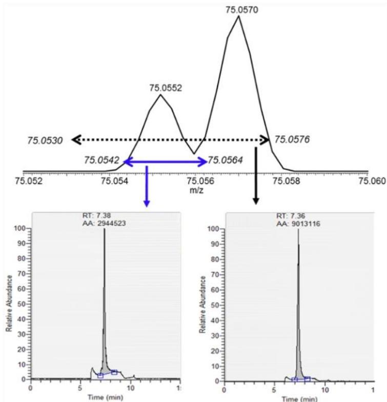
Fig. Mass spectra of Sample #13 (ER drug product) spiked with 20 ng/mL of NDMA which also contained DMF (top) and EICs (bottom) demonstrating the overestimation (integrated area of 2,944,523 with  $\pm 15$  ppm mass tolerance in the left panel (blue bar), while there is an integrated area of 9,013,116 with  $\pm 30$  ppm mass tolerance in the right panel (dotted bar)) of NDMA as the results of DMF interference from  $C_3H_7NO$
