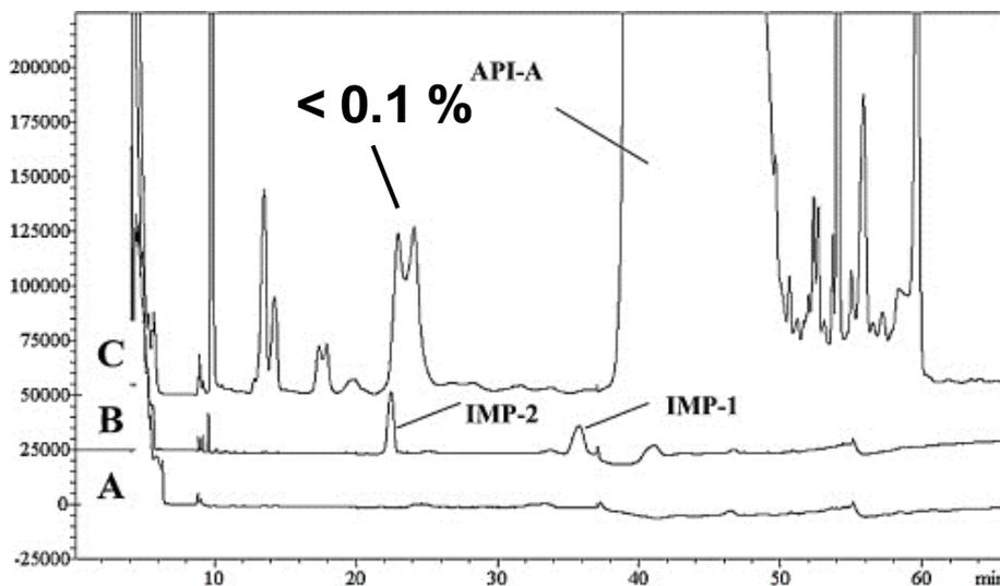
Fig. Representative HPLC chromatogram of (A) blank (DMSO), (B) IMP-1 and IMP-2 standard solution (3  $\mu\text{g}/\text{mL}$ ) and (C) API-A (40  $\text{mg}/\text{mL}$ ) in the 1st HPLC. API-A was dissolved in DMSO at 40  $\text{mg}/\text{mL}$ .
