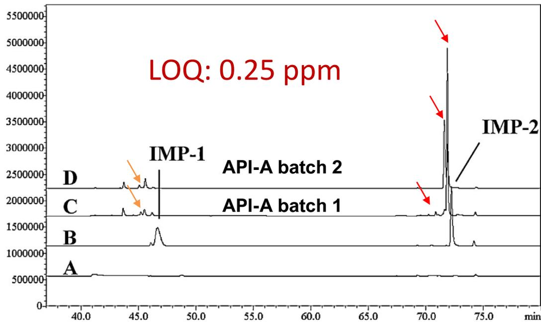
Fig. Representative HPLC chromatogram of (A) blank (DMSO), (B) IMP-1 and IMP-2 standard solution (3  $\mu\text{g/mL}$ , 75 ppm) and (C) API-A batch 1 and (D) API-A batch 2 in the 2nd HPLC.
