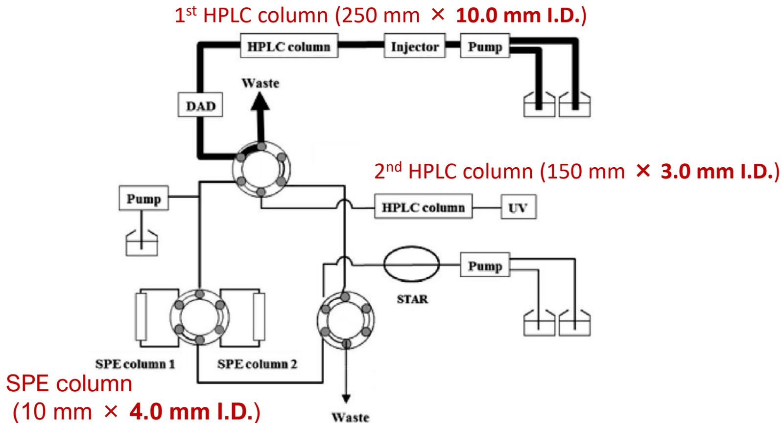
The two-dimensional HPLC system achieves a stepwise downsizing in HPLC. Trace components in the sample were concentrated, separated and subsequently detected with high sensitivity.
